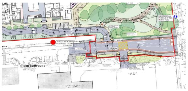
Figure 6.3 - Proposed upgrade works to existing ESB Networks facility access road
