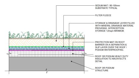
Figure 2.5 – Typical Extensive Green Roof Buildup
