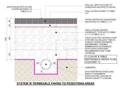
Figure 2.7 - Typical Permeable Paving Build-up
