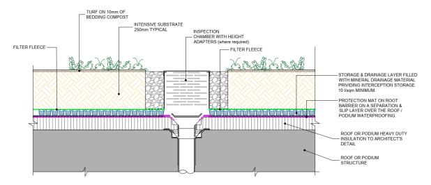
Figure 2.6 – Typical Intensive Green Roof Buildup
