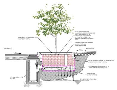
Figure 2.8 – Typical Bioretention Tree Pit Detail
